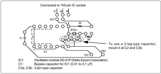
Figure 1 Oscillator circuit pattern
